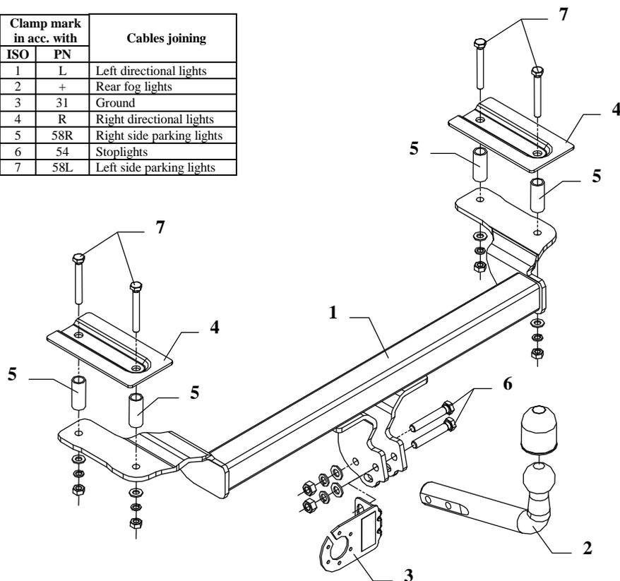
This towbar is designed to assembly in following cars: **FORD FIESTA, 3-5 doors** and **MAZDA 121 JASM/JBSM, 3 doors**, both produced since 02.1996 till 12.2001, catalogue no. **C002** and is prepared to tow trailers max total weight **950 kg** and max vertical load **50 kg**.
